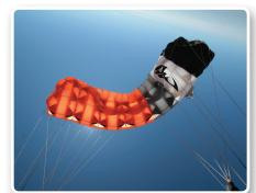
Stalling a parachute is a huge fear for most jumpers. However, exploring stalls and the slow-flight range of a canopy gives jumpers a better understanding of how their parachutes work and helps them to fly better landing patterns, improve accuracy and execute consistently soft landings.
