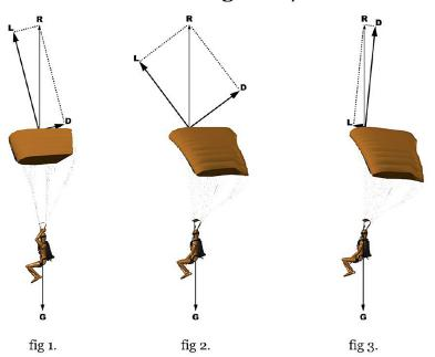
Lift and drag vectors are exaggerated for contrast.
